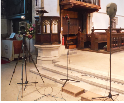
Figure 1: RIR recording set-up showing various receiver positions being recorded simultaneously for a single source position (left)
