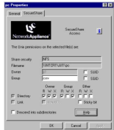
The Properties dialogue box has a new tab called SecureShare in which are the facilities to set group and world file permissions. A Help button gives access to details.
