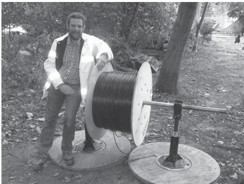
PETE TURNBULL ILLUSTRATES THE SIZE OF DRUM NEEDED FOR 2.1KM OF 48-CORE FIBRE
