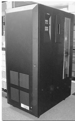
Legato is a versatile system and it would be possible to add support for other operating systems and databases, if required at a future date. Likewise the Scalar 1000 tape library can be expanded to store up to 188Tb (1 terabyte=1024Gb or 1048576Mb) of data, a figure that should comfortably accommodate the University's
