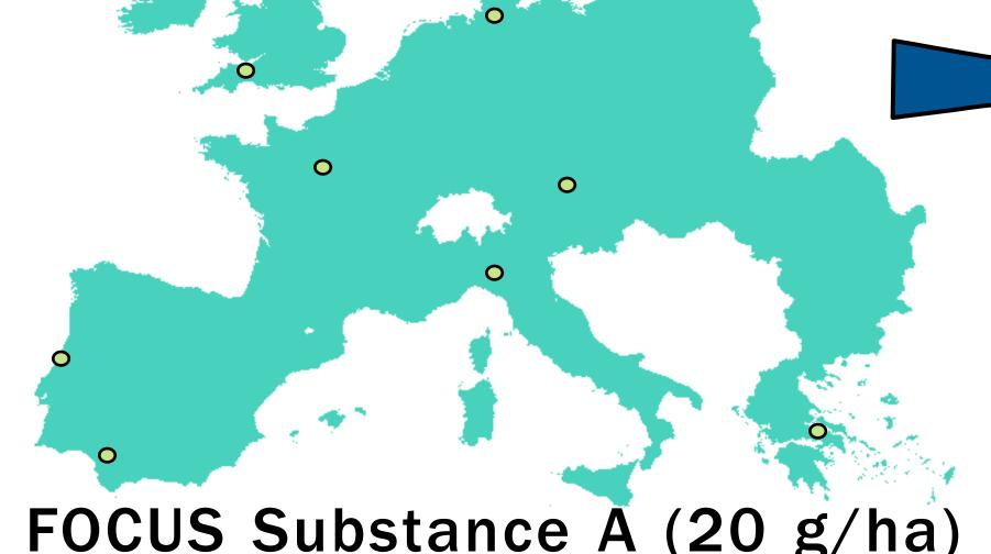
FOCUS Substance A (20 g/ha) fails application to sugarbeet at Tier 1 for scenarios C, H, K and N: PEC<sub>GW</sub>  $0.2-0.3 \mu g/L$ .
