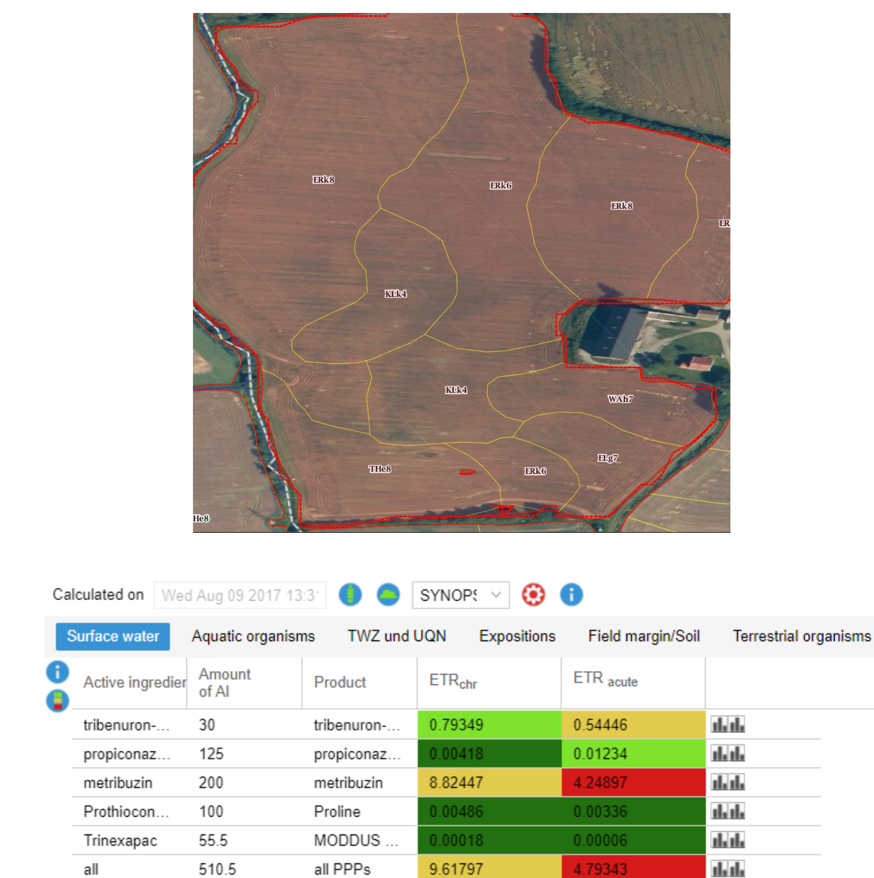
Figure 5. SYNOPSIS-WEB, an internet based tool for calculating the exposure toxicity ratio (ETR) for different field application scenarios of pesticide (Dominic et al. 2017).
