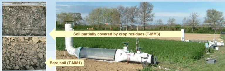
Figure 1: Wind-tunnels on bare soil (T-MM1) & on soil partially covered by crop residues (T-MM3)
