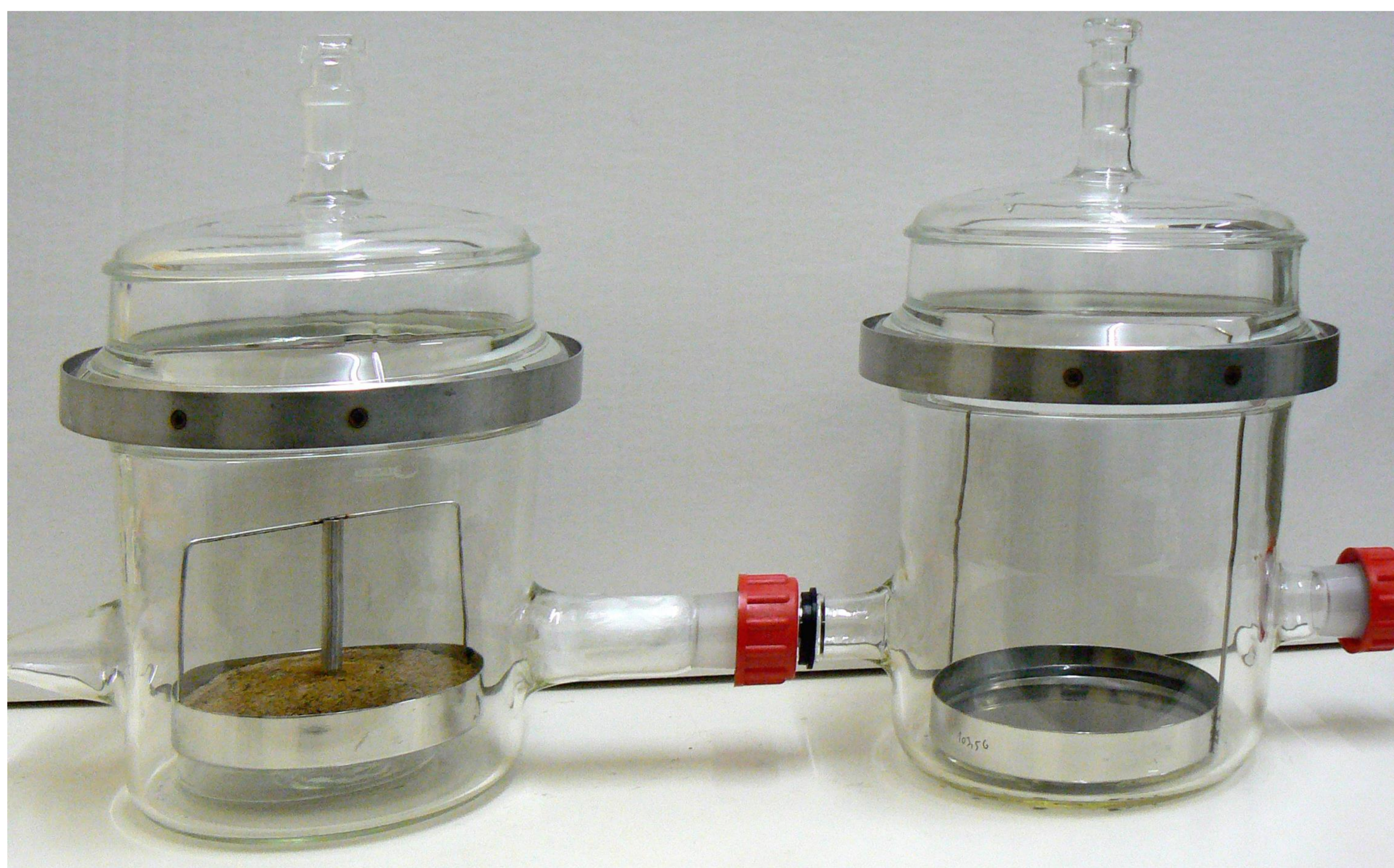
Figure 2: Volatilization chamber (left) with treated soil in petri dish and connected deposition chamber (right) with water filled petri dish.
