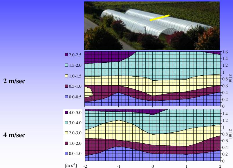
2-dimensional wind profile (cross-section along the wind tunnel)
