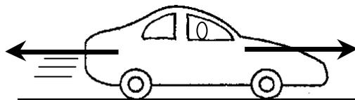
The driving force is **smaller than** the counter force.
