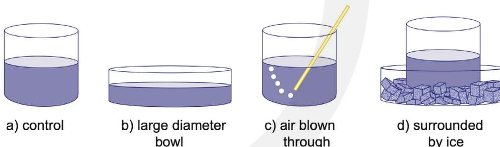
The control will show the rate of cooling due to classroom conditions, e.g. temperature. The water in b, c and d cools faster than the water in a. In b and c the water is exposed to a larger surface area of cool air (provided by air bubbles in c), and in d the water is exposed to a colder surface. Allow the children to offer explanations of their results whilst ensuring that the discussion covers the factors mentioned above.
