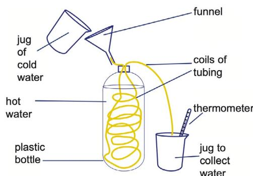
The temperature differences of the hot and cold water are compared. A space is provided on Activity sheet 14 for the children to record the differences. Typical results, with a starting temperature of 60°C, would show a rise of about 15°C for the cold water and a drop of about 5°C for the hot water.
