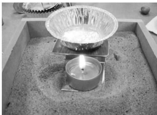
Photograph showing an oil burner heating water on a heating stand. The sand tray provides a safe area for this kind of activity.
