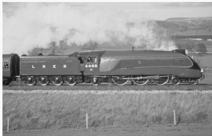
NER A4 Pacific engine of 1935 (Note that the smoke is lifted clear of the cab due to its shape.)
