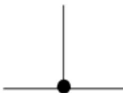
Junction (connection) between wires
