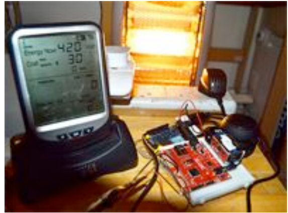
Figure 2: Testing parsing of data from an intact CurrentCost, and triggering audio tracks.
