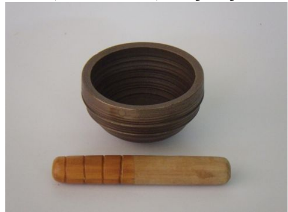
Figure 5. BP Singing Bowl 0.0, 3D printed in stainless steel.
