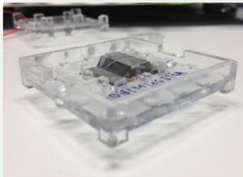
**Injection moulded waveguide chip**
