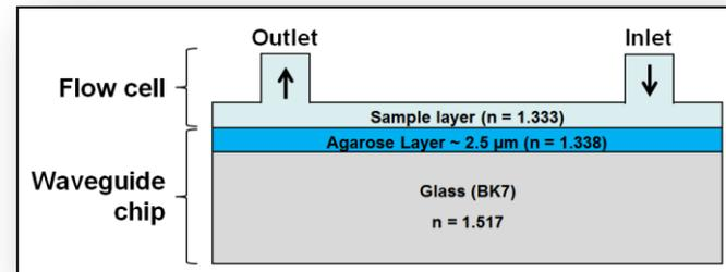
We have shown that the waveguide can detect ~2 ng mL<sup>-1</sup> alkaline phosphatase activity – this is ~15x lower than standard techniques.
