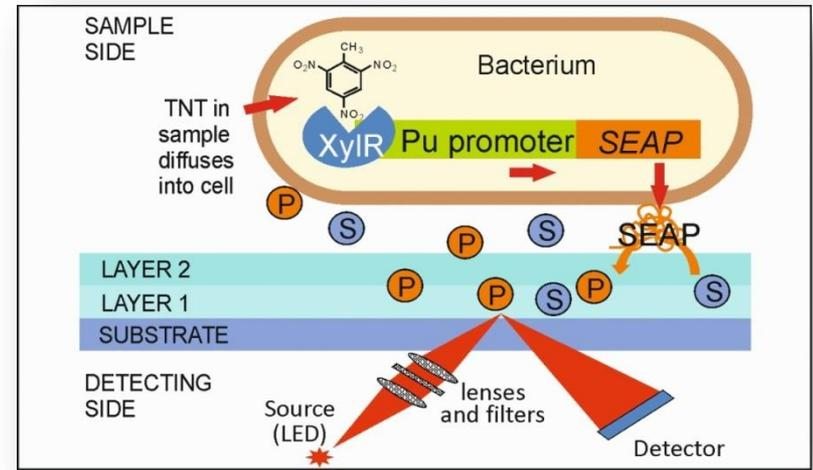
**Concept for whole-cell waveguide biosensor**
