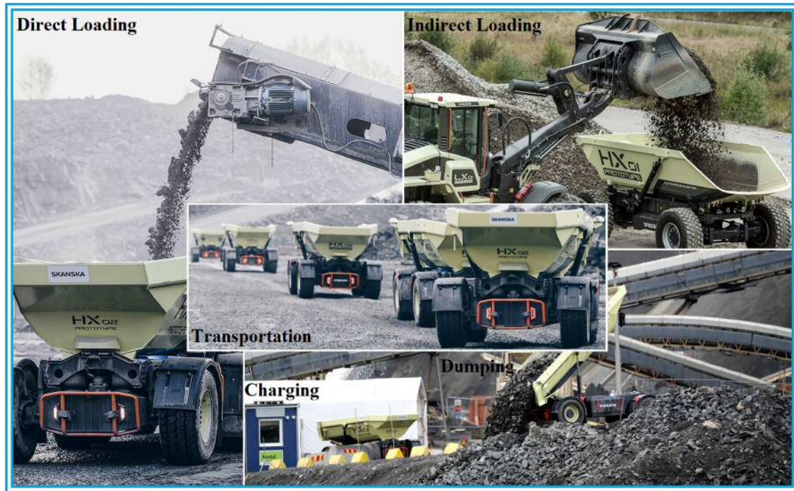
Fig. 2. Automated transportation in quarry site
