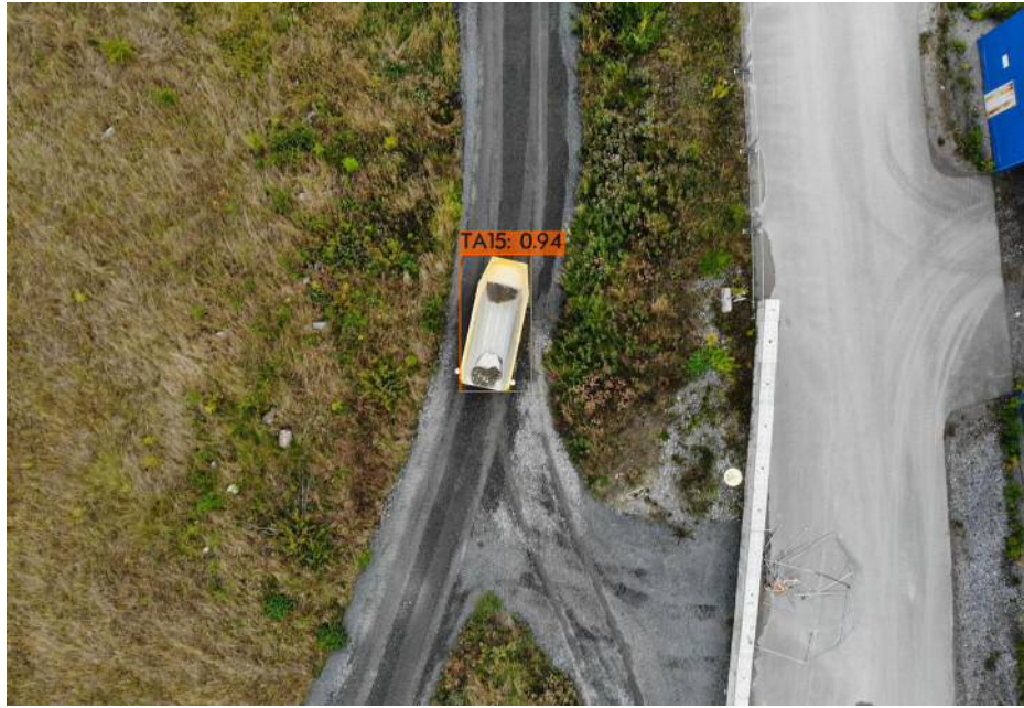
Figure 2: UAV camera picture and localizing Autonomous Machine
