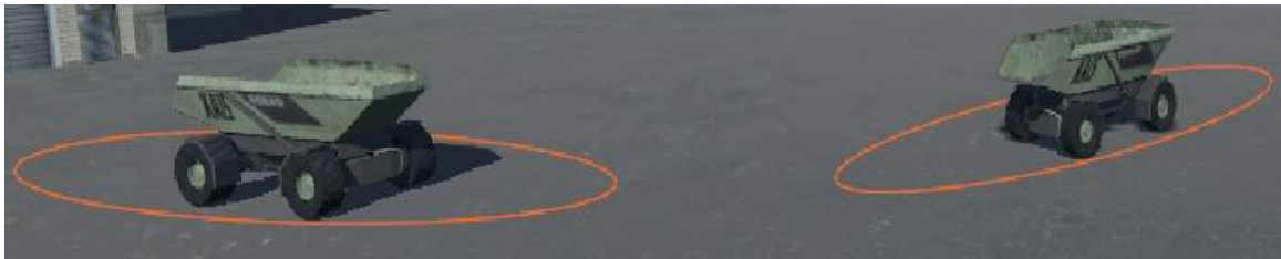
Figure 4. Capsule geometry shapes (geofences) around the haulers
