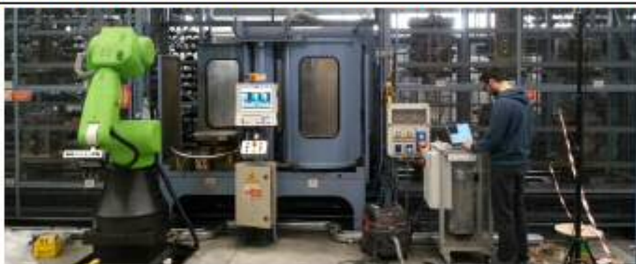
Figure 1: Front view of setup. Load/unload station used for experiments is the left one, the closed station still dedicated to manual pallet assembly. Pallets and fixtures are visible inside the automatic storage around the two load/unload stations. (Courtesy of CEMBRE S.p.A., Italy)
