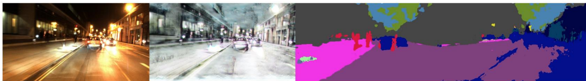
Figure 3: Instead of mapping from a difficult condition (night) to a presumed ideal condition (e.g. sunny), we learn to map from any adverse appearance to a shared, common appearance that while not seeming natural actually works better for a segmentation task.
