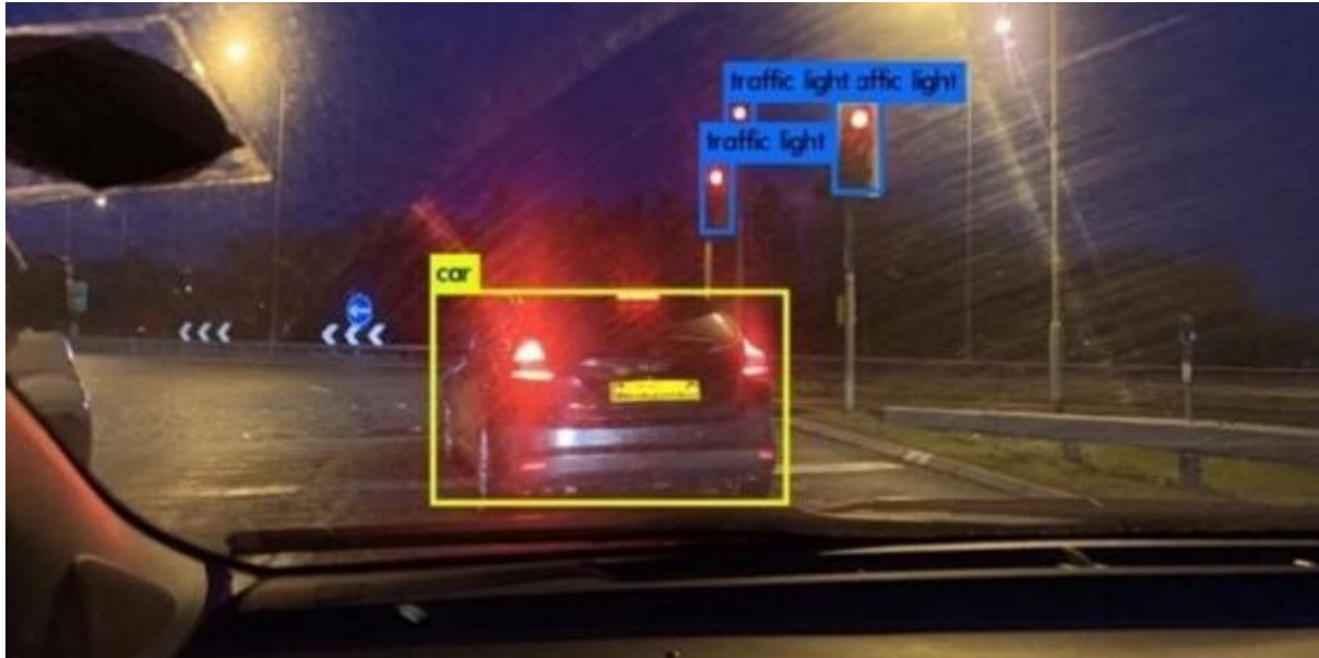
Figure 1: Example object recognition support by YOLO on public road
