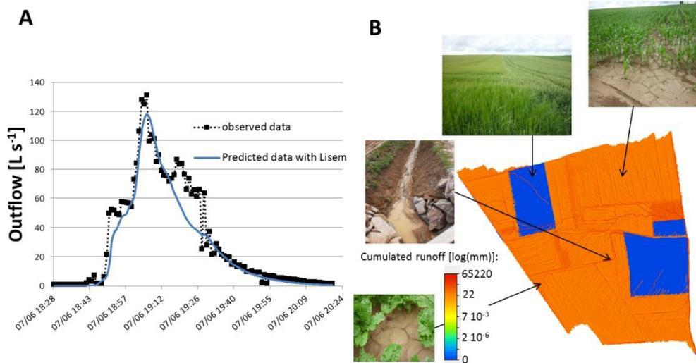
Figure 1. Simulated and observed hydrographs (A) and water pathways (B) on June 7 2012.
