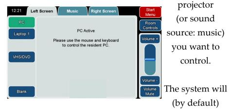
start by showing you the inbuilt PC, but you can select other sources such as DVD or laptop; or blank the screen/sound; by using the **source buttons** on the **left** of the screen. If the source has any controls, (for example DVD remote control) these will automatically appear when you select that source.
