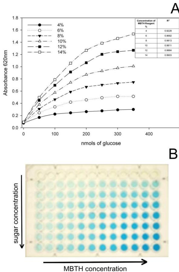
**Figure 4: Adaptation of the MBTH method for use in automated analyses (A)** Calibration curve for the detection of reducing sugars using increasing concentrations of MBTH. The insert in the figure shows the R<sup>2</sup> values obtained for the different MBTH concentrations between 0 and 200 nmol.
