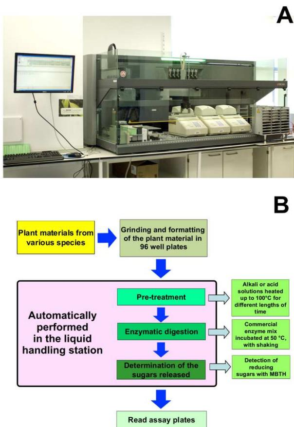
**Figure 2: Liquid handling station.** (A) General view of the liquid handling station. (B) Flow chart showing the steps involved in the saccharification analysis
