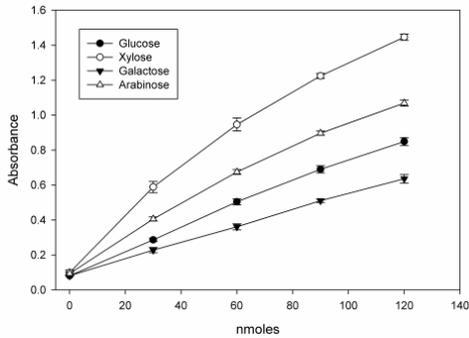
**Figure 5: Calibration curve of the MBTH detection of different monosaccharides.**
