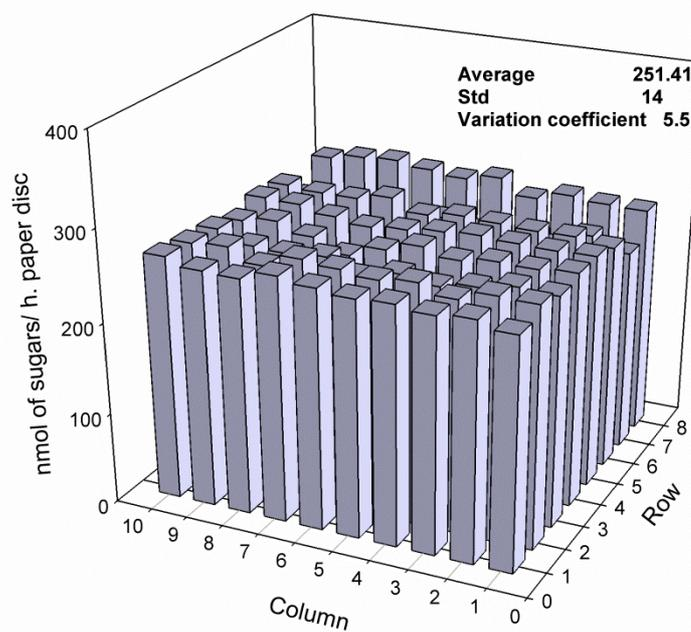
**Figure 6: Quantification of the reducing sugars released in the hydrolysis of paper discs in a 96 well plate.**
