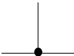
Junction (connection) between wires
