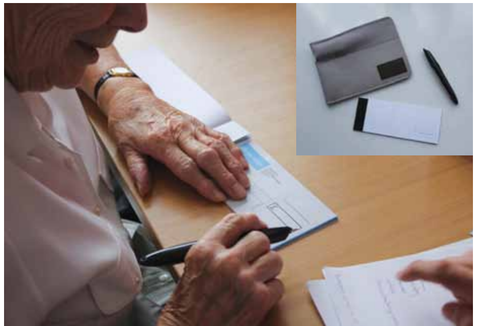
Electronic pen and cheque book – here the Anoto© pen senses what you write and transmits the information to the payment system
