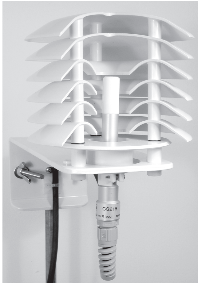
A CS215 probe shown mounted in a special cut-away version of the 41303-5 shield.
